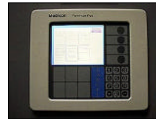
Operator interface panel with LCD display, and soft-touch keypad, in a NEMA 4X enclosure.
